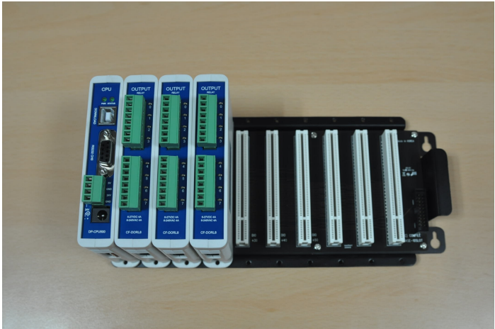
[One CPU module installed with 3 identical output modules]
