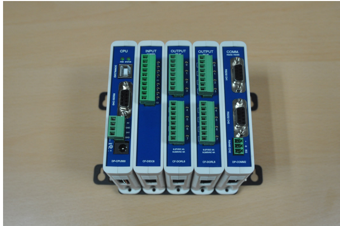
[CPU module, 3 DIO modules, and one communication module]
