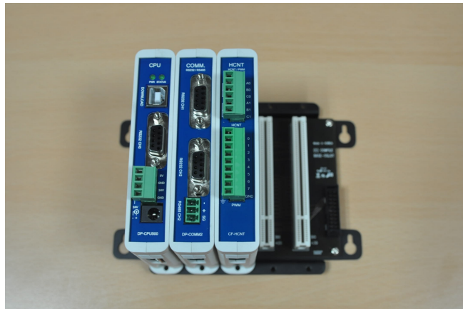
[CPU module, a high-speed counter module, and one communication module]
