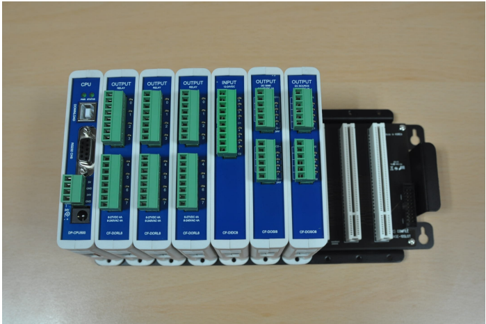
[One CPU module installed with 6 DIO modules]
