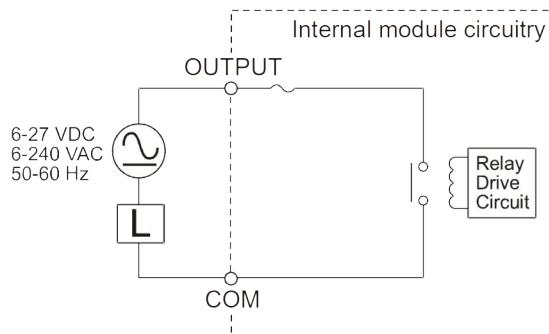
This is a 4A load per channel relay output module capable of up to AC 240V.
