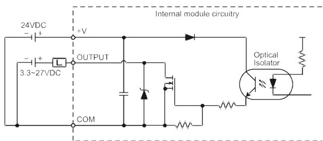
The Sink Output module requires two power sources. The DC 24V power source is used to drive the internal FET.
