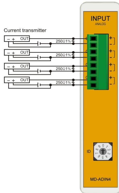
The input voltage range can be adjusted using dipswitch #2. Dipswitch #1 is not used.
