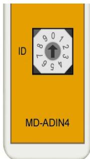
Use the rotary switch on the face of each module to set its Modbus slave address.
