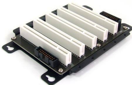
With the Header Module installed in the slot labeled "CPU", I/O modules can be installed in any of the 4 remaining slots.
