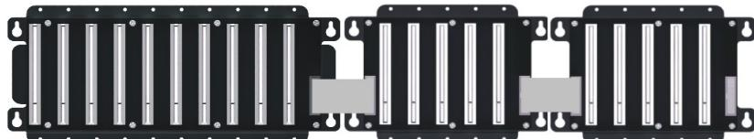
The module board array must be terminated, so if you connected additional module boards, be sure to terminate the last board in the array. A terminator is included with each board.
