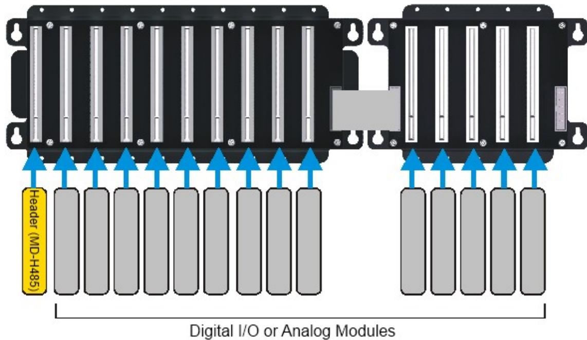
Please be sure to secure all modules to the slot board with screws.
