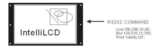
IntelliLCD can display 260,000 colors. It also supports TrueType fonts and is capable of touchpad input. It further sports additional features as follows:
