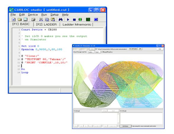
Note that the display speed of the simulator on the PC is faster than that of the IntelliLCD. This is due to the hardware difference between the PC and IntelliLCD. When you use the IntelliLCD Simulator, keep in mind that there could be other differences besides the display speed.
