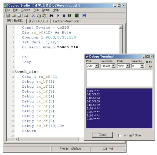
The 1st data field of the event is always 02h. Then the 2nd and 3rd fields are read to tell what kind of an event this is. (An IF statement or a Select Case statement is used.) Then the entailing data is read to determine the state of the event.
