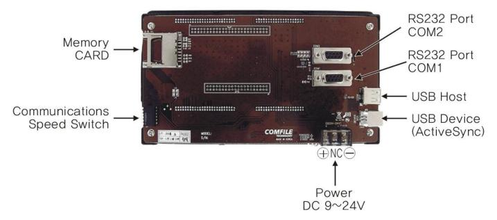
\* Make sure the polarity is correct when you connect the power to the system. Otherwise, the system may incur damage.
