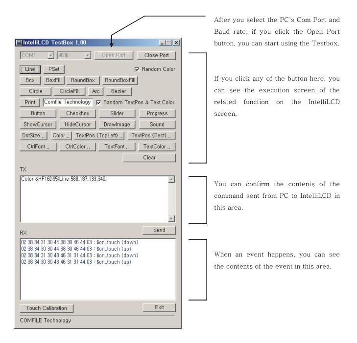
The TextBox program can also be used to check whether IntelliLCD is operating normally.
