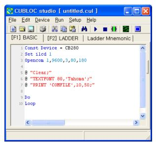
The following program is a very simple example, which displays the text string "COMFILE" on the IntelliLCD's screen.
