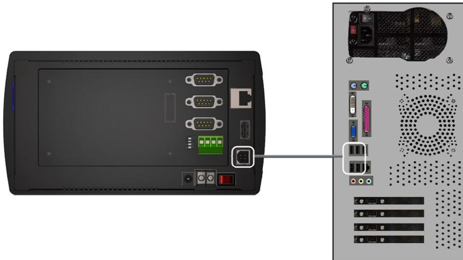
1. Once ActiveSync or Windows Mobile Device Center is installed, turn the CUPANEL on, and connect the CUPANEL touch controller to the PC with a USB Cable.
