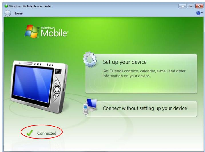
4. With the CUPANEL powered on and properly connected to the PC, ActiveSync or Windows Mobile Device Center will show a status of "Connected". The CUPANEL and the PC will then be able to communicate with one another.
