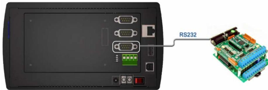
The touch controller can be connected to a PLC using any one of its three serial ports, and supports three different communication protocols: Modbus, LS Master-K (CNET), and Mitsubishi FX. The following diagrams illustrate the necessary connections that will need to be made for each of these different protocols.
