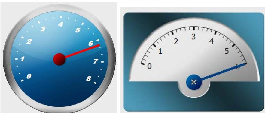
The Gauge control is analogous to the gauges commonly found on instrument panels everywhere. It is an output-only control with a rich set of aesthetic customizations.
