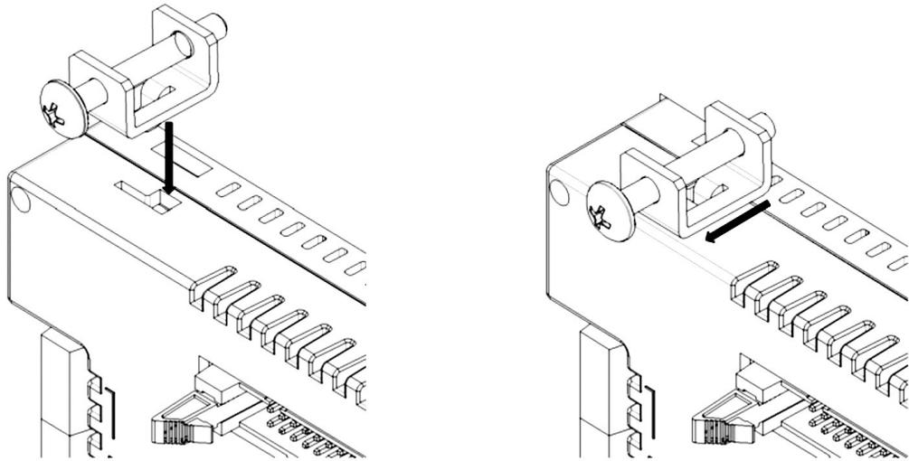
3. Slide the bracket laterally to secure in place.
