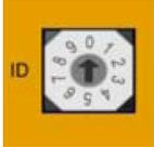
Each Modport module is assigned an ID. The ID is used to distinguish it from other modules of the same type. The ID can be assigned a number from 0 ~ 9. See the Modport manual for more information.
