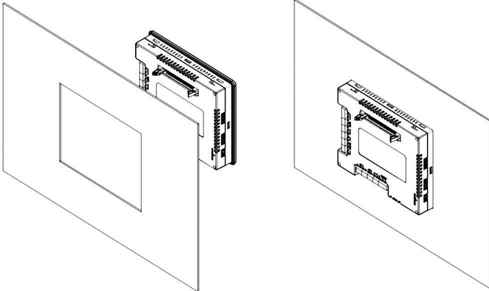
2. Insert the mounting brackets into the groove on the side of the unit, pull the bracket towards the rear of the unit.
