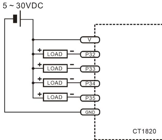
If the load is inductive, such as a relay, please be sure to connect the positive terminal to the V pin. This can help to eliminate sparking when switching.
