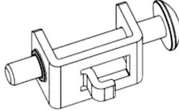
1. Insert the unit into a properly prepared panel cutout per the previously described panel cutout dimensions. (Panel thickness can be between 1 and 6 mm.)
