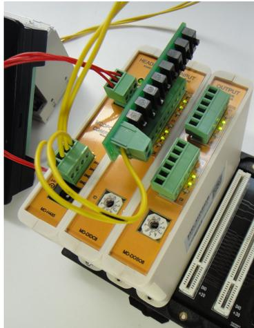
Comfile Technology's input simulator is used in this example to make it easy to toggle and test inputs. The input simulator can be purchased from <http://www.comfiletech.com/inputsimulatoer.aspx>.
