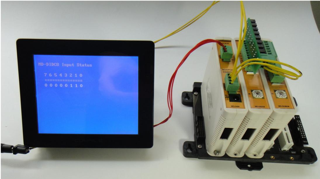
The following program reads the status of 8 inputs on the MD-DIDC8 digital module, and simultaneously outputs each status to the MD-DOS08 digital output module
