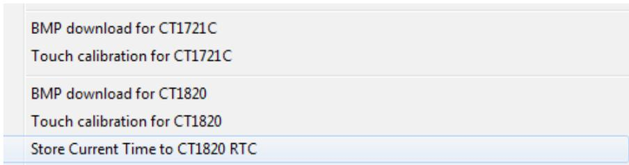
The CT18XX series' RTC is battery powered, so in between power cycles, the RTC's date and time continue to increment. However, the RTC is not 100% accurate, and if used for an extended period of time, a drift may become apparent, and will need to be re-synchronized with a current time source.
