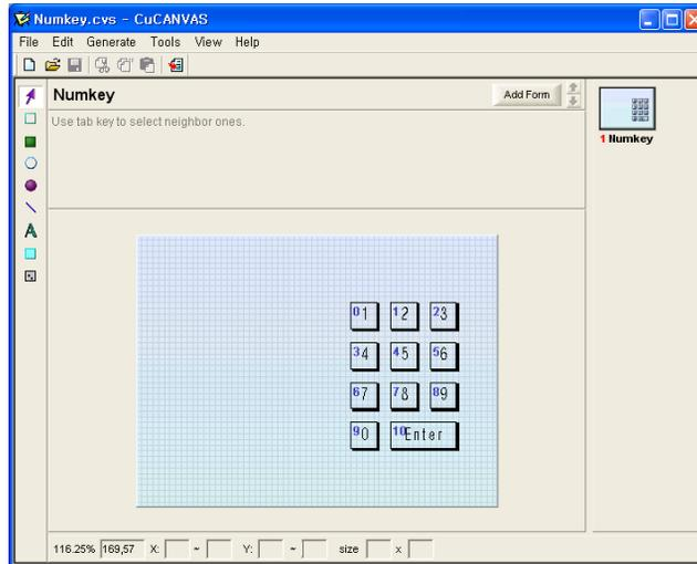
Select the "View/Hide Code" button from the top toolbar to show the generated BASIC code. As shown below. Click the "To Clipboard" button to copy the code and paste it in "Cubloc Studio".
