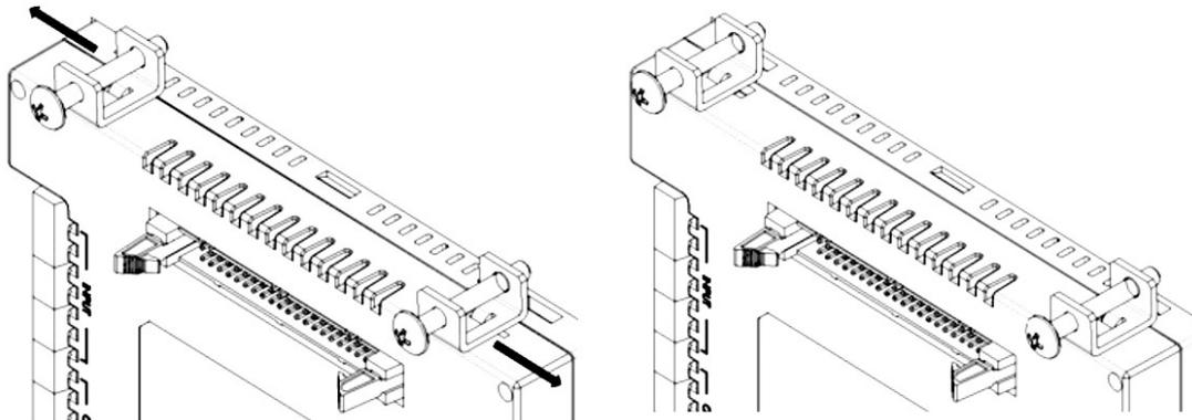
4. Tighten the bolts to secure the unit to the panel.
