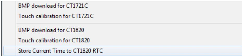
In Cubloc Studio's "File" menu, there is a "Store Current Time to CT1820 RTC" menu option. This feature can be used to set the CT1820's RTC's date and time to that of the PC running Cubloc Studio.
