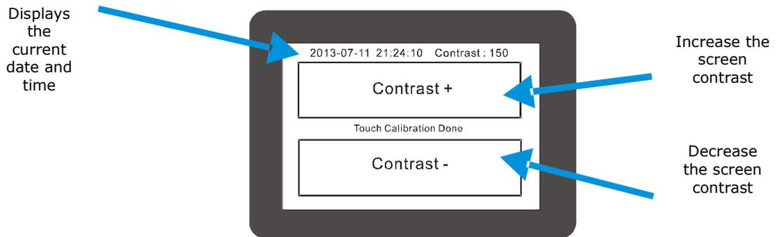
Each CT1820 will have to have its contrast set individually. It can be set at runtime using the CT18Contrast command as shown below.
