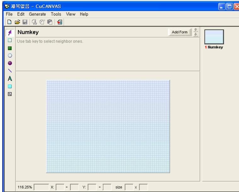
The toolbar on the left can be used to draw boxes, circles, lines, etc.. Click the "Menu for CUTOUCH" button to add a menu button. After clicking the button, draw the button on the screen.
